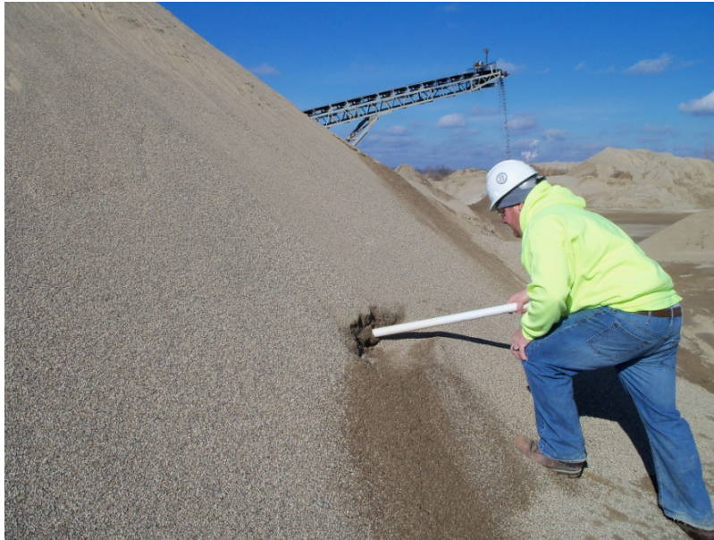
Using a Sand Tube for Natural Sand
